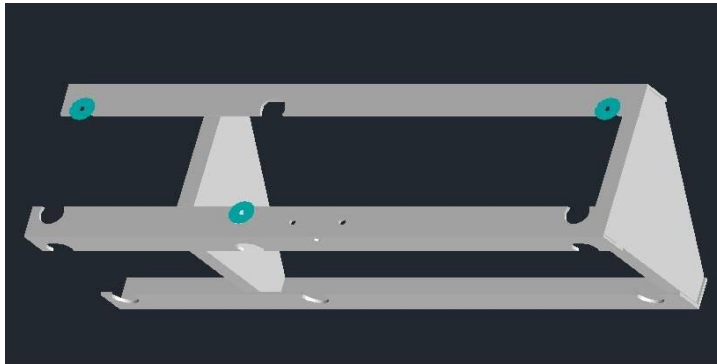
Test Bar with Retros / CAD plot: Allows different numbers and configurations of retro-reflectors
